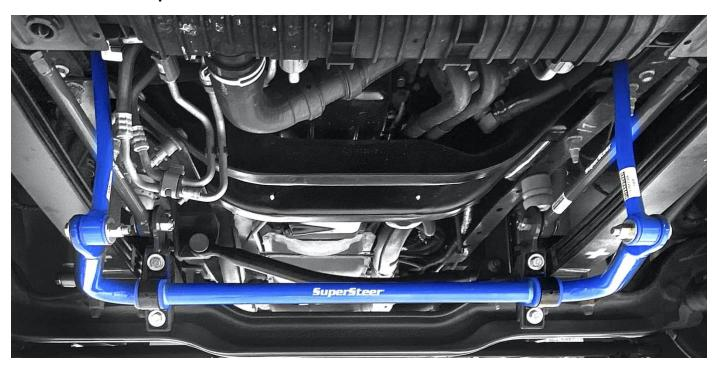
MARNING: The SS-101 sway bar is not a load-bearing component
