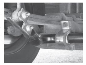
MARNING: Loosening the saddle bracket bolts will release the sway bar. The sway bar is heavy, and may cause property damage or personal injury if it falls on equipment, engine components or any part of your body. Ensure that the sway bar is supported and that you are out of the way when removing the bolts. Failure to follow these instructions may cause property damage.
